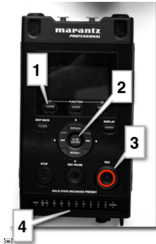
Figure 6. The Marantz PMD-661. 1) The F1 button; 2) Enter button; 3) Record button; 4) LED levels meter.
