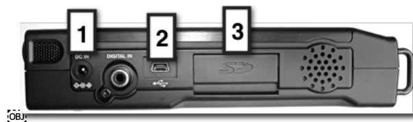
Figure 7. Left side view of the Marantz PMD-661. 1) DC-in power jack (for plugging the unit into a wall plug); 2) USB port; 3) SD card compartment.
