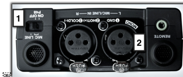
Figure 3. Top view of the Marantz PMD-661. 1) Phantom power selector; 2) XLR input jack for the microphone.
