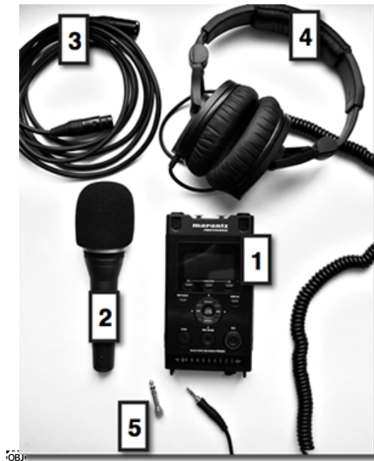
Figure 2. Recording equipment. 1) Marantz PMD-661; 2) AKG D5 mic; 3) XLR cable; 4) Sennheiser headphones; 5) 1/8"-to-1/4" headphone plug adapter.
