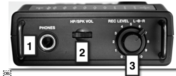
Figure 4. Bottom view of the Marantz PMD-661. 1) Headphone jack; 2) Headphone volume adjuster; 3) Recording level control knob.
