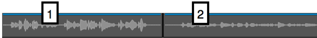
Figure 8. Waveforms of recorded audio. 1) Levels were set correctly; 2) Levels were set too low
